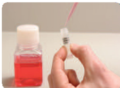
Figure 3. Reconstitution of MitoXpress Intra reagent
